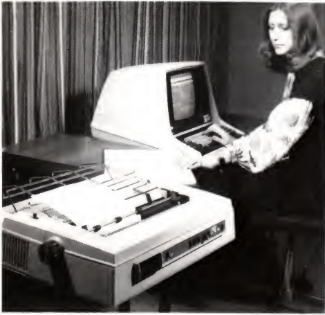
The word processor. This microcomputer doubles as an accounting system and a word processor. Foreground – a high quality printer prints out a letter.
